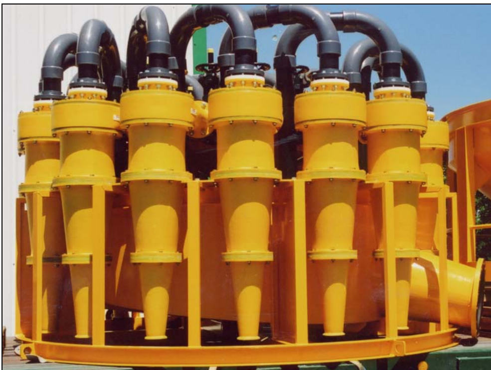
Batterie de 16 hydrocyclones HB 280 (Ø 280 mm) Cluster of 16 hydrocyclones HB 280 (Ø 280 mm)
